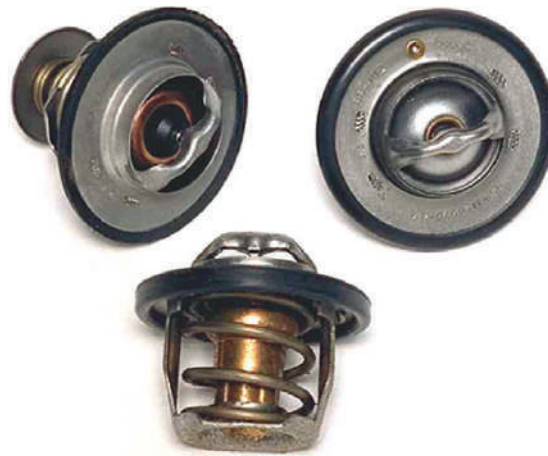
Figure 2.154 Thermostat with its wax pellet in the hot-coolant area
